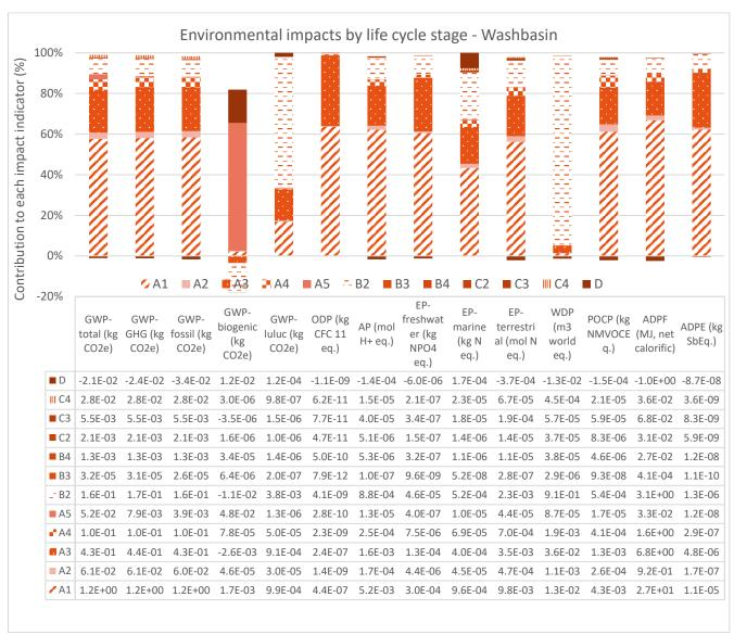
The raw materials suply is the largest source of GHG emissions, accounting for 59 % of the GHG impact (A+B+C). Of all the raw materials, the resin is the most impactful.
