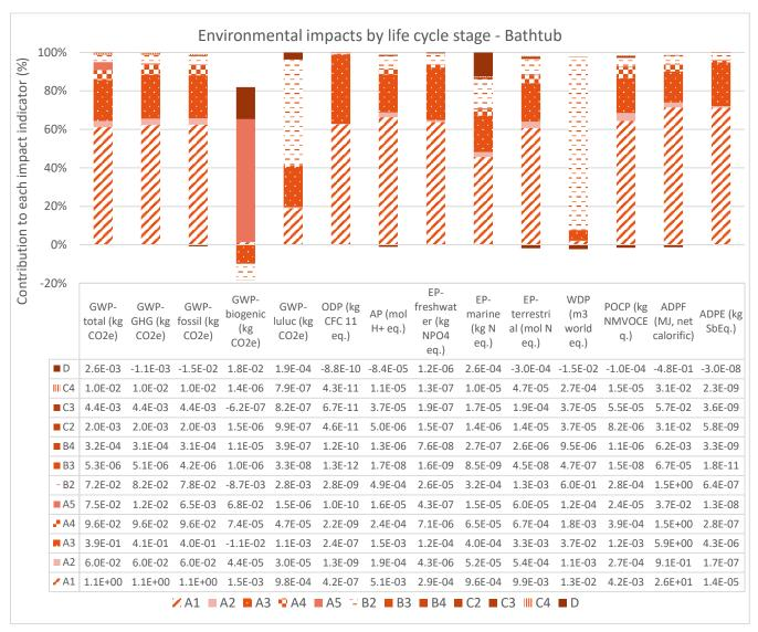
The raw materials acquisition is the largest source of GHG emissions, accounting for 62 % of the GHG impact (A+B+C). Of all the raw materials, the resin is the most impactful.
